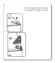
3. Remove screws 1 and hinge 2.
