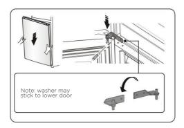
15. Move the upper door to an appropriate position, and then fix part 2 by screws 1.
